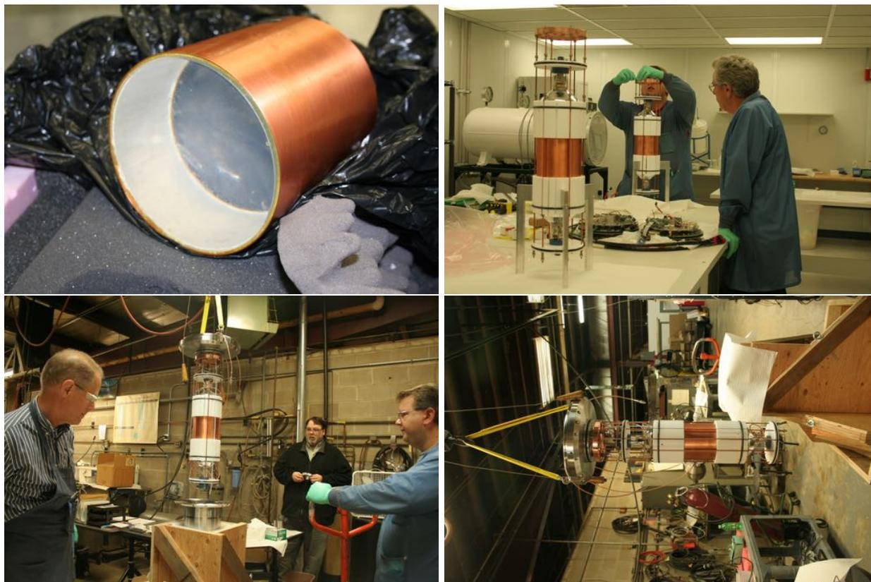
**Figure 5.8:** Assembly of the DM-Ice17 detectors. Clockwise from top left: NaI(Tl) crystals from the NaIAD experiment arrived in Wisconsin in September 2010; the detectors were assembled in September and October 2010 at PSL by first coupling the crystals, light guides, and PMTs; the mainboards were added to the top of the detector; the assembly was placed inside stainless steel pressure vessels and loaded into the shipping containers for transport to the South Pole.
