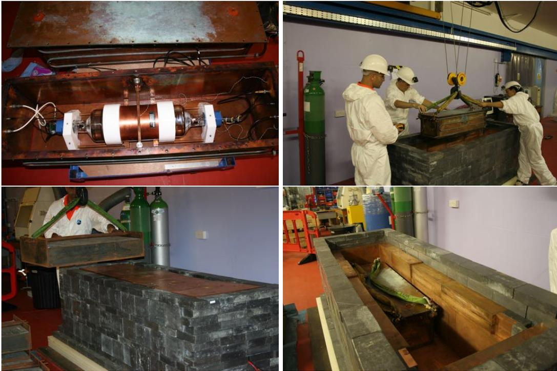
**Figure 6.7:** Setup of Boulby calibration testing. Images, clockwise from top left: one of the copper-encapsulated crystals coupled to PMTs on either end; lowering a crystal into the lead castle; the lead castle setup with the crystal inside; covering the lead castle.
