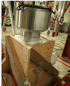
**Figure 6.9:** Setup of PSL calibration runs. The detector was in its final configuration and already in the shipping crate. The  $^{207}\text{Bi}$  source can be seen taped to the shipping crate on the right hand side.
