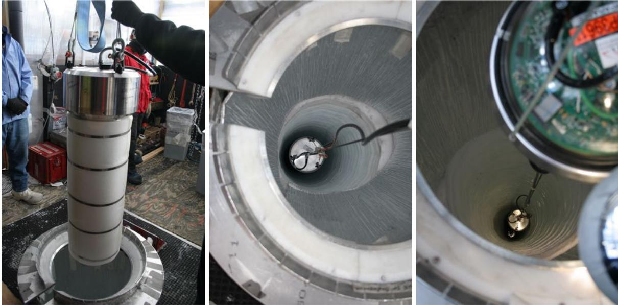
**Figure 5.11:** Deployment of DM-Ice17 Det-2. It was wrapped in an additional layer to further protect against thermal shock. The right-hand figure shows an IceCube module entering the hole directly above Det-2.
