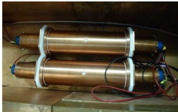
**Figure 5.3:** DM-Ice37. Two 18.7 kg NaI(Tl) crystal are deployed at Boulby for R&D. Testing of crystal and PMT contamination are underway to determine the feasibility of currently available components for the full-scale detector. The crystals are housed in a lead castle and continuously flushed with nitrogen.
