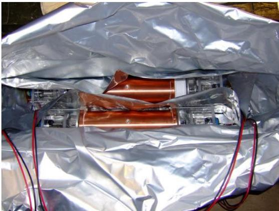
(b) DM-Ice test crystals in mylar bag
